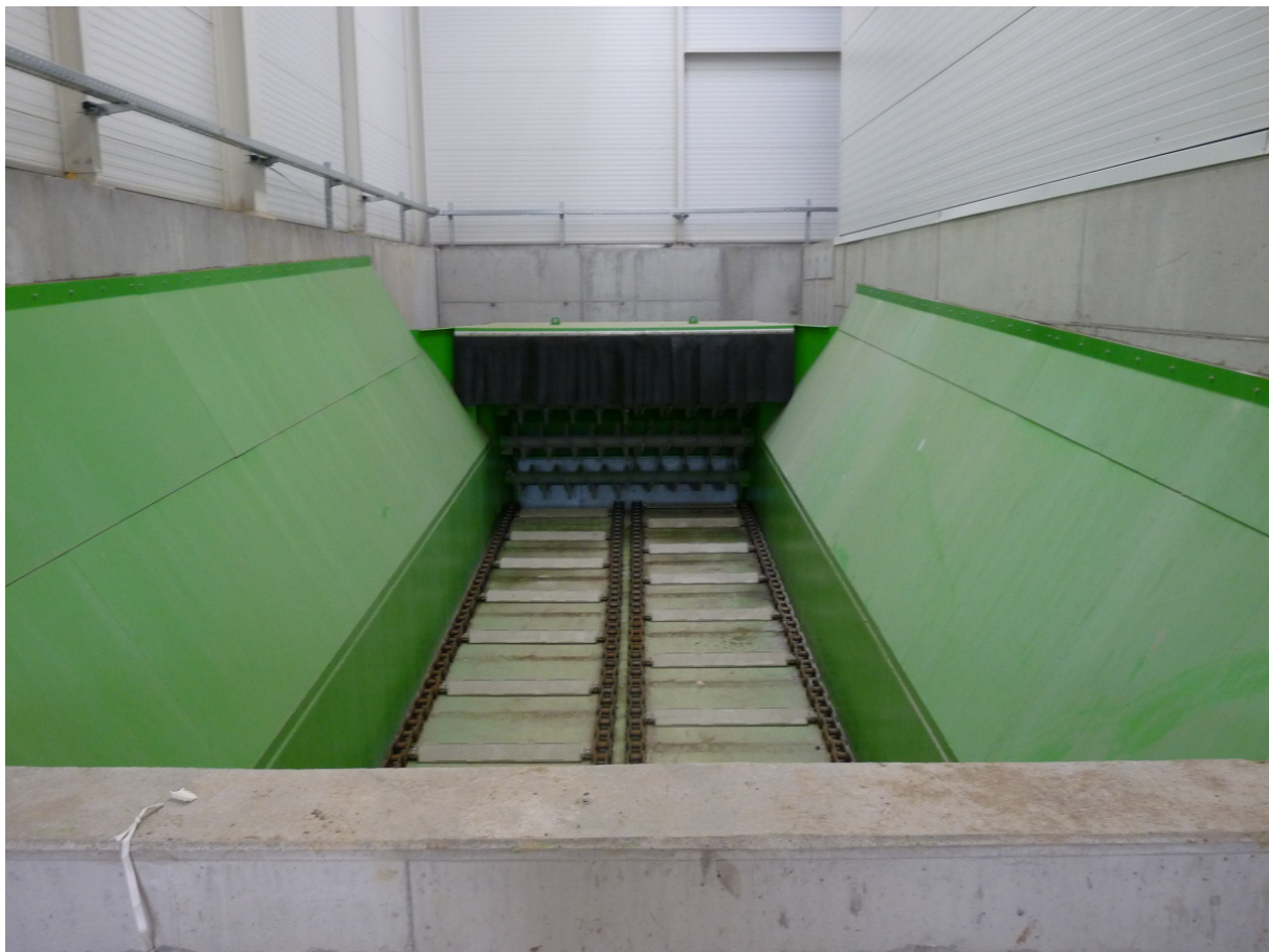
Fig. 4.11: Poultry dung reception hopper
