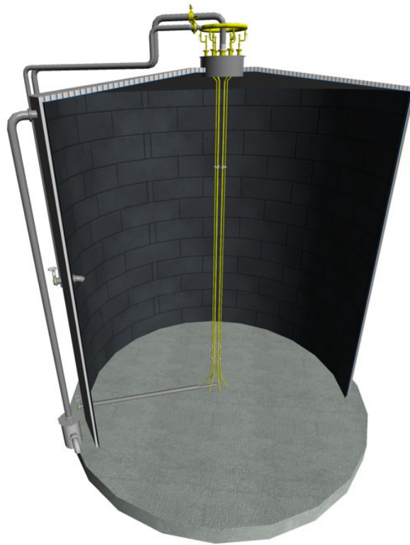
Fig. 4.13: Scheme of gas lances from gas mixing system
